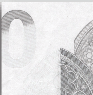
IR-light proves banknote's IR response
